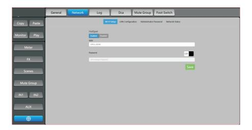
5. Select Wi-Fi Setup option to enter wireless network setup page. You can set hotspot name and password.
