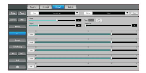
12. Select FX tab, got to effect control page, choose different effect module for control, and choose dispatch and control dispatch amount. reverb effect and delay effect.
