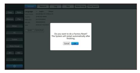
7. Restore system default settings Select Factory Reset button, or press and hold UBOOT (hidden on the back) for more than 3 seconds while the computer is on. Select OK to restore default settings and Cancel to abort the restoration.
