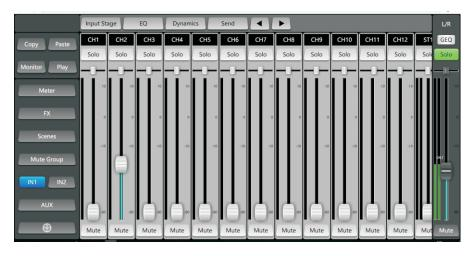
1. Channel main page (go to system's first page) take DM16 mixer as an example. The page displays channel status and button to go to the subpage. Click button to enter the corresponding subpage menu.
