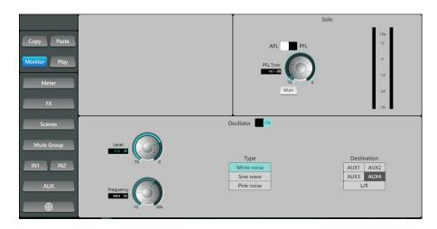
Select Monitor tab, go to monitor control and Oscillator signal generator controller page.
