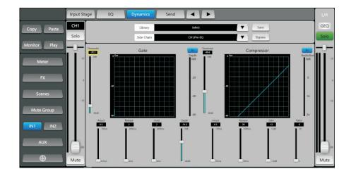
7. Select Dynamics tab, go to Dynamics control page. Adjust noise gate and compression parameters.
