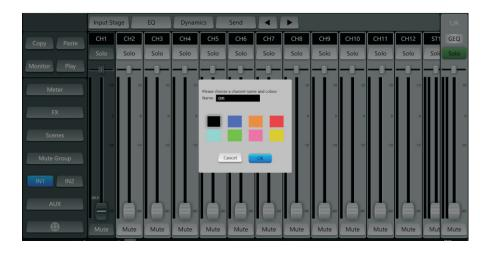
4. You can modify the name and color of CH1 channel by clicking the position of CH1 with the mouse. For modifications to other channels, click the appropriate channel position. The left and right arrows can move to the left or right for channel selection.
