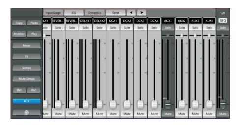
3. Select AUX tab, the right window displays as shown in the picture. Channel selection can also be dragged with the mouse to display.
