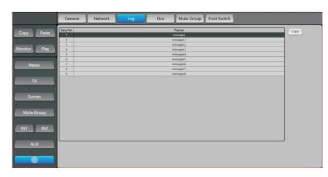
17. Select log option to enter system log page, which saves the last 10 boot records, use Copy button to copy the log information to an external USB flash disk (requires inserting a USB flash disk).
