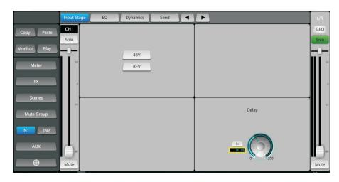
5. Select Input Stage tab, go to input channel settings page, current channel 48V, REV (phase) and Delay parameters can be controlled.
