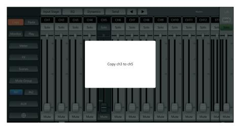
14. Copy/Paste function, set parameters in current channel, and after finishing click copy, choose other channels, click paste, can copy channel parameter settings.
