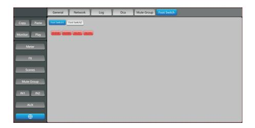
20. Select Foot switch tab, got to foot switch configuration page. Can set the corresponding module for foot switch control.
