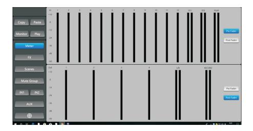
11. Select Meter tab, go to whole level table display page. Indicates whole signal level and can select signal indication before and after fader.
