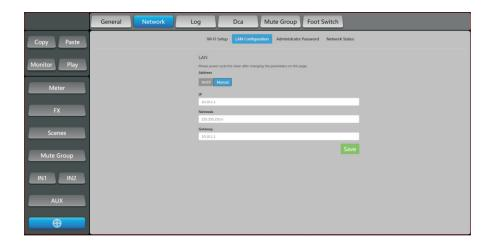
3. Select LAN Configration settings, go to wired network settings page. You can view the device IP address, or manually change the IP. Under the same network, type this IP in the connected control device (PC) browser to connect and control the device.
