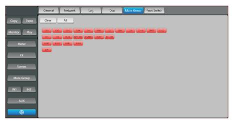
19. Select Group Setup tab, go to grouping configuration page. Default mute grouping configuration is for mute all, settings can be changed as needed.
